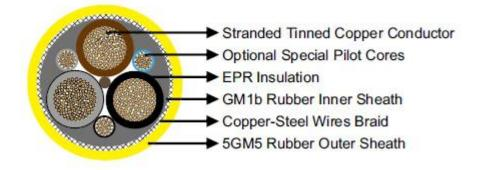
**Conductors:** Flexible stranded tinned copper conductor, class 6 according to DIN VDE 0295. **Insulation:** EPR.
