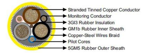
**Conductors:** Flexible stranded tinned copper conductor. **Insulation:** Heatresistant3GI3 rubber based on EPR.
