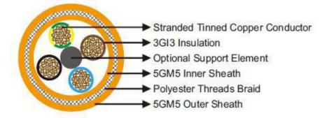
Conductors: Flexible stranded tinned copper conductor.
